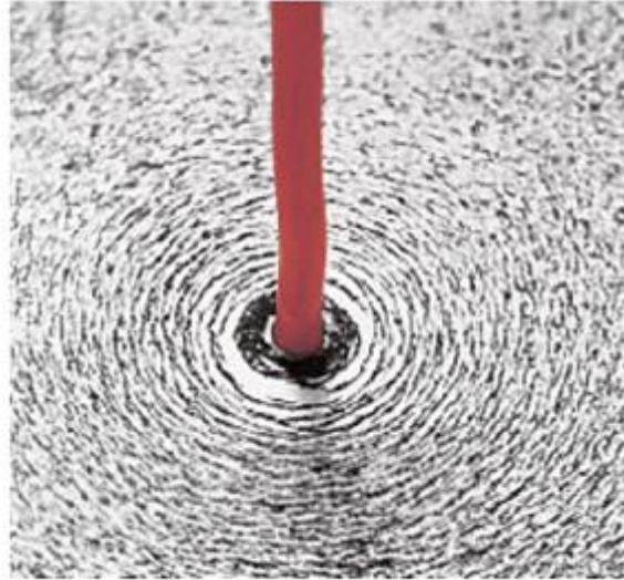
Magnetic Field Around a wire
