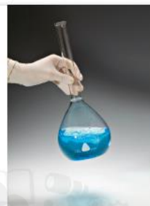
Step 2: The solute is placed in a volumetric flask of the correct volume.
