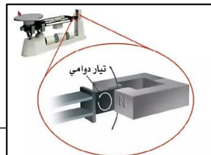
Figure 11 As the metal plate on the end of the balance beam moves through the magnetic field, an eddy current is generated in the metal. The eddy current produces a magnetic field that opposes the motion that caused it. This dampens the beam's oscillations.
