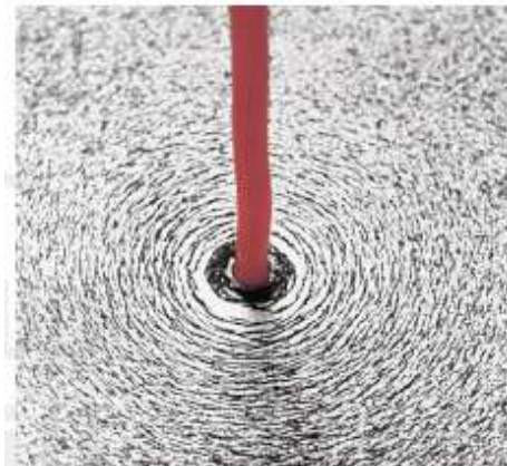
Magnetic Field Around a Wire
