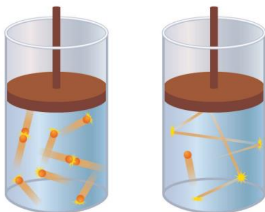
Figure 2 Kinetic energy can be transferred between gas particles during an elastic collision. Between collisions, the particles move in straight lines.
