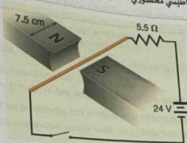
▪ Determine the magnitude and direction of the magnetic force on the wire when the switch is closed.
