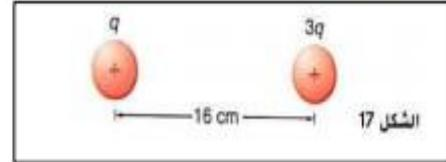
$$q_B = 3 q_A =? \quad r_{AB} = 16 \text{ cm} = 16 \times 10^{-2} \text{ m} \quad F_{AB} = 0,28 \text{ N}$$
