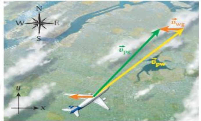
FIGURE 3.19 Velocity of an airplane with respect to the wind (yellow), the velocity of the wind with respect to the ground (orange), and the resultant velocity of the airplane with respect to the ground (green).
