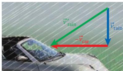
FIGURE 3.21 The velocity vector \vec{v}'_{\text{rain}} of rain, as observed from inside the moving car.
