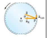
**EXAMPLE 8–5** Angular and linear accelerations. For the child on the rotating carousel of Example 8–4, determine that child's (*a*) tangential (linear) acceleration, (*b*) centripetal acceleration, (*c*) total acceleration.
