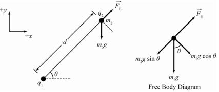
**RESEARCH:** The repulsive force between two charged beads is  $F_{\rm E} = k \frac{q_1 q_2}{d^2}$ . Using Newton's Second Law,
