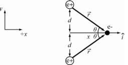
**RESEARCH:** By symmetry the forces in the vertical direction cancel. The force is therefore due solely to the horizontal contribution  $F \cos \theta$  in the  $\hat{x}$  direction: the Coulomb force is  $F_{21} = kq_1q_2 / r_{21}^2$ .
