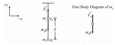
**RESEARCH:** The electric force on  $q_2$  is given by  $F_E = kq_1q_2/d^2$ . The gravitational force on  $m_2$  is  $F_g = m_2g$ .
