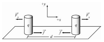
**RESEARCH:** Assume the surface is parallel to the surface of the Earth. The frictional force is  $f = \mu N$ , where N = mg. The electrostatic force is  $F = kq^2 / d^2$ . The beads will start to move as soon as F is greater than f, enabling one bead to move away from the other. Then the minimum charge q can be found by equating f and F.
