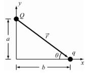
**RESEARCH:** The electrostatic force is  $F = kqQr/|r|^2$ . The *x*-component of this force is  $F_x = (kqQ/r^2)\cos\theta$ . The values of b for which  $F_x$  is a minimum can be determined by inspection; the values of b for which  $F_x$  is a maximum can be found by calculating the extrema of  $F_x$ , that is, taking the derivative of  $F_x$  with respect to b, setting it to zero, and solving for b.
