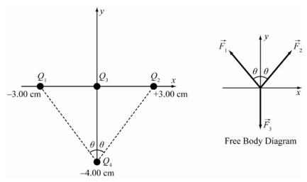
**RESEARCH:** The magnitude of the forces between two charges,  $q_1$  and  $q_2$ , is  $F = kq_1q_2 / r^2$ . The forces on  $Q_4$  are
