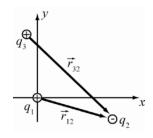
**RESEARCH:** The magnitude force is  $\overrightarrow{F_{12}} = kq_1q_2\hat{r}_{12} / |\overrightarrow{r_{12}}|^2 = kq_1q_2\overrightarrow{r_{12}} / r_{12}^3$ . The net force on  $q_2$  is the sum of all the forces acting on  $q_2$ .
