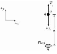
**RESEARCH:** The electrostatic force on the mass *m* is  $F_E = kq^2 / d^2$ . This force is balanced by the gravitational force  $F_g = mg$ . Therefore,  $F_E = F_g \text{ or } kq^2 / d^2 = mg$ .
