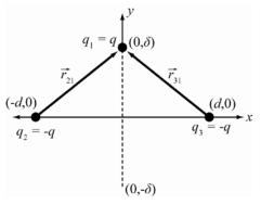
**RESEARCH:** The Coulomb force is  $\overrightarrow{F_{21}} = kq_1q_2\hat{r}_{21}/r_{21}^2$ , where  $\overrightarrow{F_{21}}$  is the force on the charge 1 by charge 2, and  $\hat{r}_{21}$  points from charge 2 to charge 1. To first order, the binomial expansion is, in general,  $(1+x)^n \approx 1+nx$  for  $x \ll 1$ . The restoring force of a simple harmonic oscillator obeys Hooke's Law,  $F = -\omega^2 mx$ , where  $\omega$  is the characteristic angular frequency, and  $f = \omega/(2\pi)$ .
