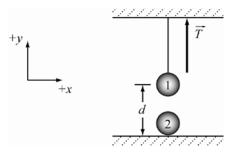
**RESEARCH:** The electrostatic force between two charges is  $F = kq_1q_2/r^2$ . The force of gravity is  $F_g = mg$ . The ball will leave the floor if the electrostatic force between the two balls is greater that the force of gravity, that is if  $F > F_g$ , and if the charges are opposite. The tension in the rope can be found by considering all of the vertical forces acting on the first ball.
