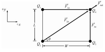
**RESEARCH:** The magnitude of the force between two charges is  $\vec{F}_{12} = \left(kq_1q_2 / |\vec{r}_{21}|^2\right)\hat{r}_{21}$ . The total force on a charge is the sum of all the forces acting on that charge. The magnitude of the force is found from  $F = \left(F_x^2 + F_y^2\right)^{1/2}$ , where the components  $F_x$  and  $F_y$  can be considered one at a time.
