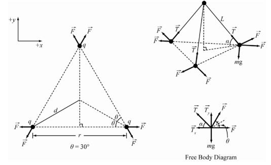
**RESEARCH:** The magnitude of the force between two charges,  $q_1$  and  $q_2$ , is  $F_{12} = kq_1q_2/r^2$ . The magnitude of F in the above figure is  $F = kq^2/r^2$ . Using Newton's Second Law, it is found that  $T_y = T \sin \alpha = mg$  and  $T_x = T \cos \alpha = 2F \cos \theta$ .
