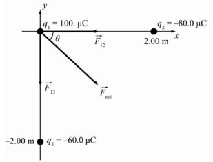
**RESEARCH:** The magnitude of the force between two charges is  $F = k |q_1| |q_2| / r^2$ . The net force on  $q_1$  is
