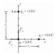
**RESEARCH:** The magnitude of the force between two charges is  $F = k |q_1| |q_2| / r^2$ . The net force on  $q_1$  is  $\vec{F}_{net} = \vec{F}_{12} + \vec{F}_{13} = -\frac{k |q_1| |q_2|}{r_1^2} \hat{x} - \frac{k |q_1| |q_3|}{r_2^2} \hat{y}$ . The direction of the net force is  $\theta = \tan^{-1} \left( \frac{F_y}{F_x} \right)$ . **SIMPLIFY:** Not needed
