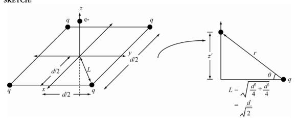
**RESEARCH:** The electrostatic force between two charges is  $F = kq_1q_2 / r^2$ . By symmetry, the net force in the horizontal direction is zero, and the problem reduces to a balance of the forces in the vertical direction, with one fixed charge balancing a quarter of the electron's weight. The vertical component of the electrostatic force is  $F \sin \theta$ . The weight of the electron is  $W = m_e g$ .
