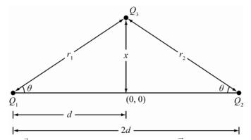
$\vec{F} = \vec{F}_{13} + \vec{F}_{23}$ , where  $\vec{F}_{13}$  is the force  $Q_3$  feels due to  $Q_1$  and  $\vec{F}_{23}$  is the force  $Q_3$  feels due to charge  $Q_2$ . Because  $Q_1$  and  $Q_2$  have the same sign and are of equal charge there is no net force in the horizontal direction. The forces due to  $Q_1$  and  $Q_2$  in the vertical direction are given by:
