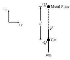
The attractive force between the cat and the metal plate is  $F = kQQ/d^2$ . Since the cat is suspended in the air, this means that F = mg. Therefore  $mg = kQ^2/d^2$ . Solving for Q gives  $Q = \sqrt{mgd^2/k} = d\sqrt{mg/k}$ . Substituting m = 7.00 kg,  $g = 9.81 \text{ m/s}^2$ ,  $k = 8.99 \cdot 10^9 \text{ N m}^2/C^2$  and d = 2.00 m yields
