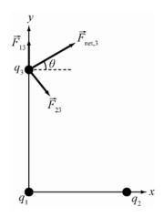
**ROUND:** With 2 significant figures in each given value, the final answers should be rounded to  $\vec{F}_{\text{net,3}} = (2.265 \cdot 10^{-5} \text{ N})\hat{x} + (1.568 \cdot 10^{-5} \text{ N})\hat{y} = 2.8 \cdot 10^{-5} \text{ N}$  and  $\theta = 35^{\circ}$ .
