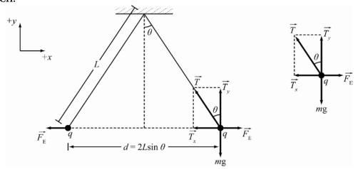
**RESEARCH:** The force due to electrostatic repulsion of the two spheres is  $F_{\rm E} = kq_1q_2 / d^2 = kq^2 / d^2$ . Applying Newton's Second Law yields (I)  $T_x = T\sin\theta = F_{\rm E}$  and (II)  $T_y = T\cos\theta = mg$ . L = 0.45 m,  $m = 2.33 \cdot 10^{-3}$  kg,  $\theta = 10.0^{\circ}$ .
