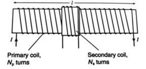
26- If the current in the primary coil decreases uniformly from 12.0 A to zero in 58.0 ms and the  $(\Delta V_{ind})$ induced in the secondary coil is 8.03 V, calculate the mutual inductance, M.
