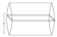
Let x represent the distance measured (in ft) from the bottom of the tank, as shown in the above diagram. The entire tank corresponds to the interval  $0 \le x \le 3.281$  (as 1 mt = 3.281 ft). Let us partition the tank into
