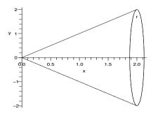
Consider a line  $y = (\frac{r}{h})x$  Rotating it about the x-axis, we get a cone of radius r and height h Here
