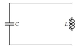
The capacitor is fully charged using a 18.0-V battery and is then connected to the circuit.
