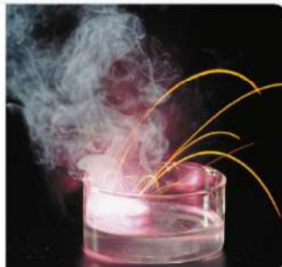
Figure 3 Potassium metal reacts vigorously with water, releasing so much heat that the hydrogen gas formed in the reaction catches fire.
