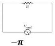
**Single-loop circuit with a resistor and a source of time-varying emf**
