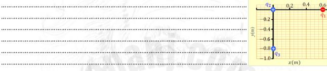
In the figures below, three-point charges are placed in a space If the net electric force on charge (q1) is zero where (q2=+4 $\mu$ C) and (q1=-2 $\mu$ C), find the magnitude of charge q3.
