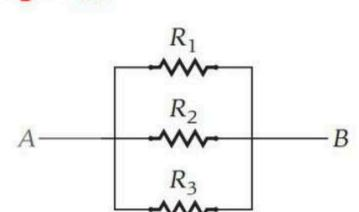
Which combination of resistors has the highest equivalent resistance?
