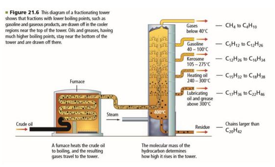
■ Figure 21.7 Fractional distillation towers separate large quantities of petro-leum into usable components. Thousands of products we use in our homes, for transportation, and in industry result from petroleum refining.
