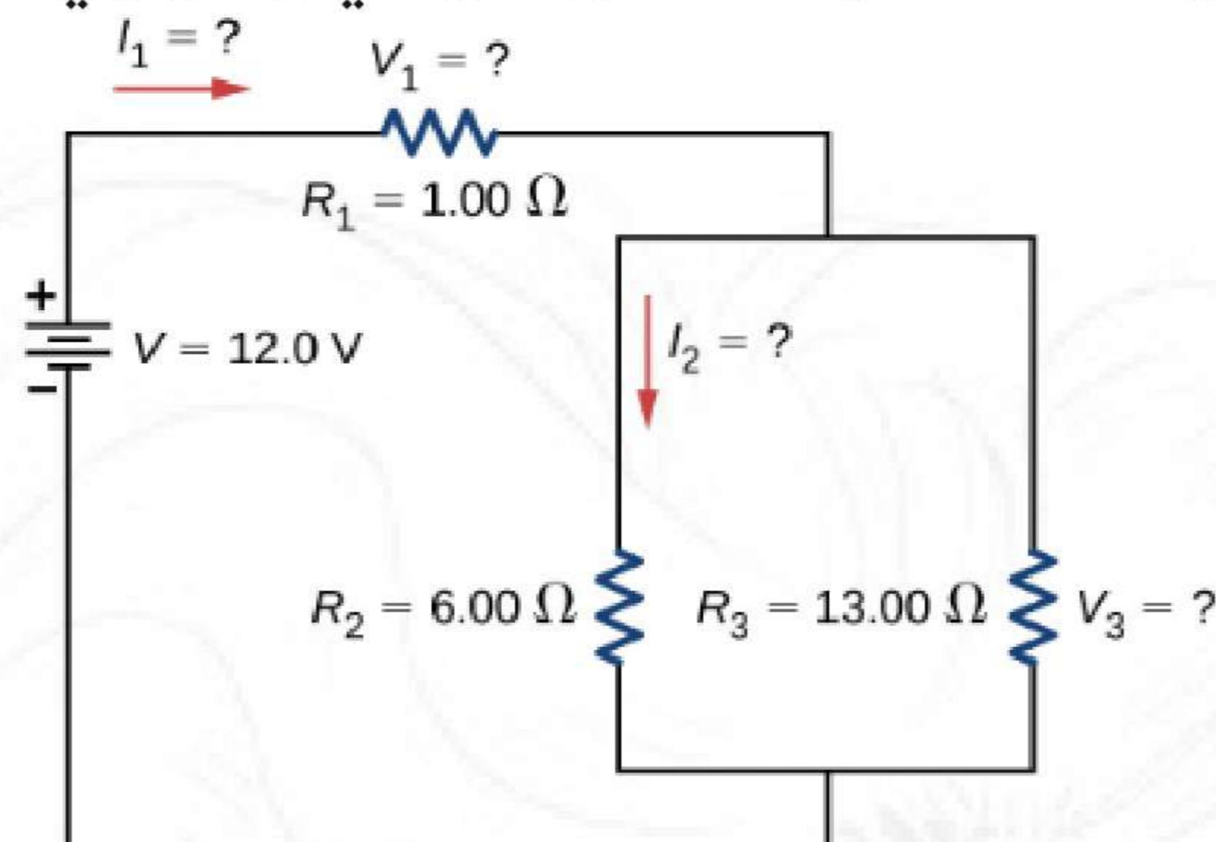
Find the equivalent resistance of the circuit.
