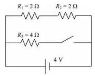
What is the current flowing in the circuit initially, when the switch is open?
