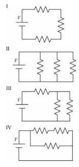
Which of the circuits will have the same voltage, V, across each one of its resistors?
