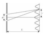
Light with wavelength  $\lambda$  is incident on two narrow slits spaced d meters apart. An interference pattern is visible on a screen located L meters from the slits. The second dark fringe is observed to be x meters from the prominent central maximum. The diagram above shows the path of light rays extending from each slit to the second dark fringe. What it the path difference?
