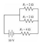
How much heat is generated in the 4  $\Omega$  resistor in 2 seconds?
