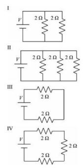
Which of the circuits will dissipate the most power?
