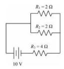
What current will flow through the  $4 \Omega$  resistor?
