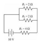
What is the voltage drop around the 4  $\Omega$  resistor?
