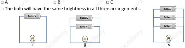
13) Identical batteries are connected in three different arrangements to the same light bulb as shown in the figure. Assume that the batteries have no internal resistance. In which arrangement will the bulb shine the brightest?
