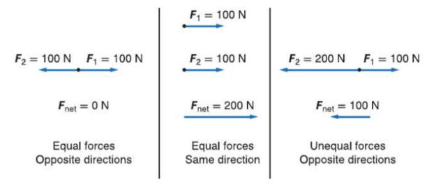
When the net force  $F_{net}=0$  there is no acceleration (balanced system, equilibrium)
