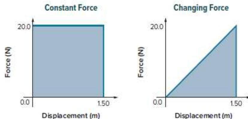
Figure 4 The area under a force-displacement graph is equal to the work.
