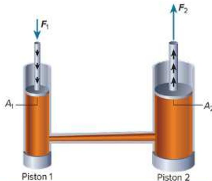
**Figure 10** As  $F_1$  exerts pressure on the smaller piston (piston 1), the pressure is transmitted throughout the fluid. As a result, a multiplied force ( $F_2$ ) is exerted on the larger piston (piston 2).
