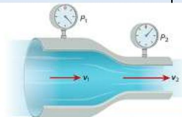
**Figure 15** The fluid flowing through this pipe also demonstrates Bernoulli's principle. As the velocity of the fluid increases ( $v_2$  is greater than  $v_1$ ), the pressure it exerts decreases ( $P_2$  is less than  $P_1$ ).
