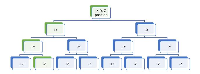
The probe should always try to maintain the position to 0,0,0 from the orbit. That is why when the value of X position is (+) positive, the system will reduce X by 1 each time.
