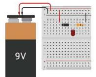
The status of the LED depends on whether the diode was connected correctly or not. It must be connected in the direction that allows the current to flow through it.
