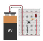
If the circuit constructed properly, when the students press the pushbutton the LED should turn on.
