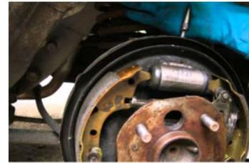
Slave cylinders are mounted to the back – plate on a drum brake system
