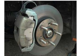
A slave cylinder is incorporated into the brake caliper on a disc brake system
