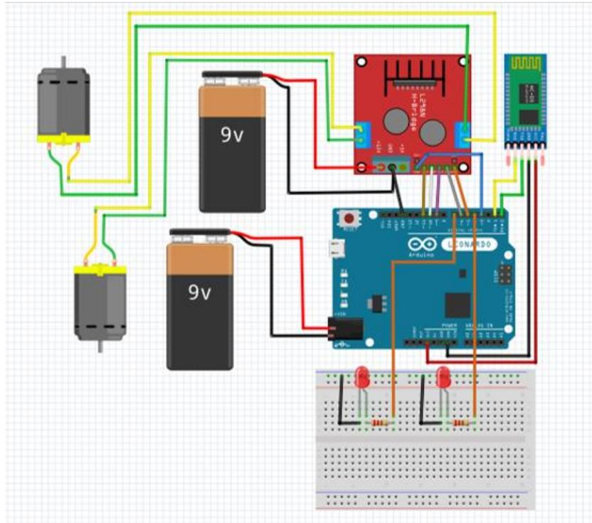
Figure 4.1.27: Simulation diagram for a space rover with headlights
