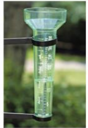
A rain gauge measures how much rain has fallen.
