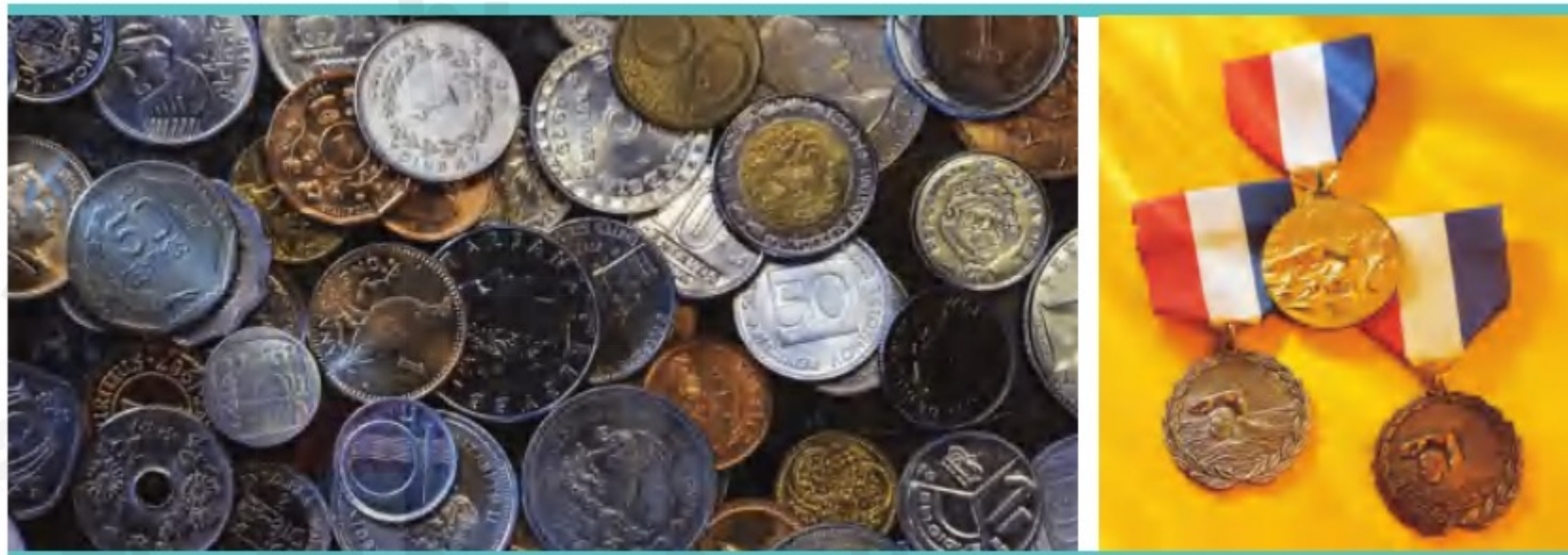
Figure 7 Copper is often mixed with zinc or nickel to make modern coins. Gold, silver, and bronze—an alloy of copper and tin—are used to make athletic medals.
