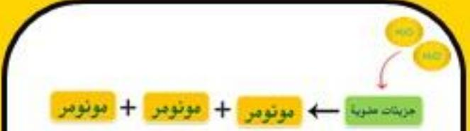
The diagram illustrates the hydrolysis of a polymer. At the top right, two yellow circles labeled 'H<sub>2</sub>O' are shown. Red arrows point from these circles to a green box labeled 'جزيئات مائية' (Water molecules). Below this, a green arrow points from the 'جزيئات مائية' box to a sequence of three yellow boxes labeled 'مونومر' (Monomer), separated by plus signs. This represents the breakdown of a polymer into its constituent monomers.
